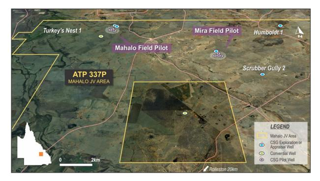
The objective of the Mahalo and Mira pilot schemes is to lift water from the coal seams, which reduces the pressure in the area around the wells and allows gas to flow to the wells. Ultimately the aim for either
